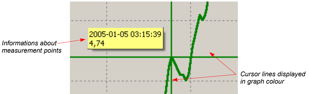
Fig. 3.9. Graph with special tracking cursor
