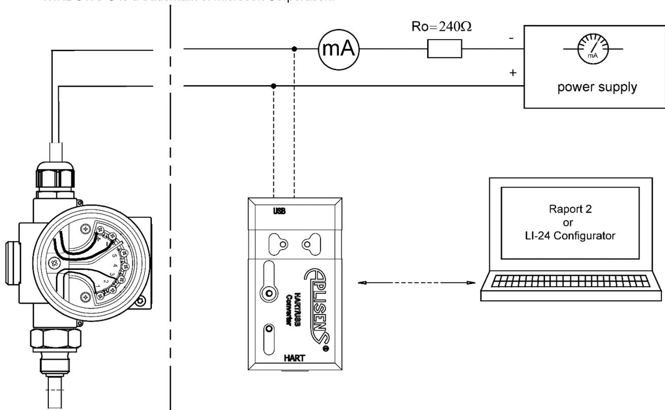
**Fig. 1.** Diagram of transmitter connection to the current loop for testing.
