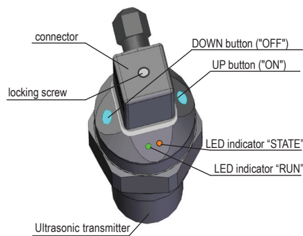
Fig. 29: Key parts of the measuring device (version with buttons)
