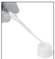
4. Add contents of pipette to the bottom chamber. Repeat once, adding a total of 3 shots of water to the bottom chamber.
