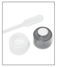
1. If the above conditions in the "Inspection Prior to Recharging" section are met, you may recharge your EasyCare CalCheck® chamber(s). Follow the procedure outlined in the "Initial Charging" section.
