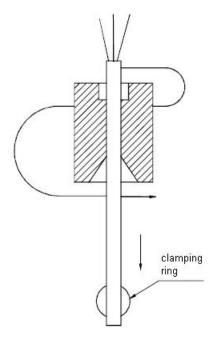
In order to mount the weight onto the cord, put the cord through the whole of the weight and rotate the weight to break away the clamping ring. Next, slide the clamping ring onto the cord at the desired spot and put the weight onto it, so that the weight is blocked on the cord. Make sure to connect power supply with power voltage disconnected from the device, following the attached diagram. Once power supply is connected, check the connection and insulation of live clamps.
