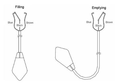
At minimum level the contacts 'black – blue' are shorted (release condition). When the liquid level in tank rises, the contacts 'black – blue' remain shorted until maximum level is reached. Once maximum level is reached, snap action switching occurs, the contacts 'black – blue' break and the contacts 'black – brown' are shortened. They remain shortened until the float reaches minimum level.
