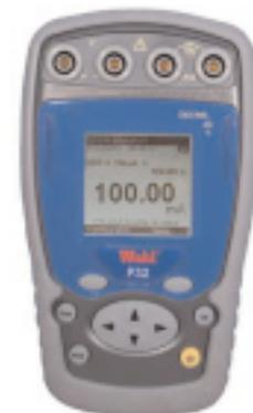
Fully configurable scaling with units: User can also program scaling in accordance with the sensor or transmitter with unit changing: 4-20mA output signal from a 0-100 bar transmitter will be measured by P32 with bar display and reading between 0 and 100 bar.
