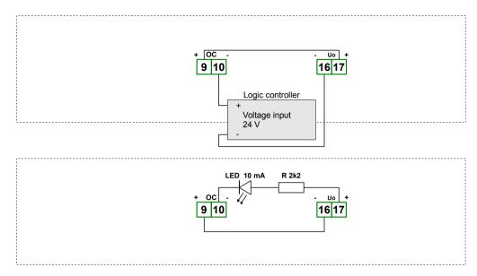
Figure 4.17. Example of OC-type outputs connection
