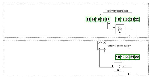
Figure 4.12. Connection of 3-wire current converters
