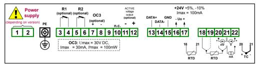
Figure 4.10. Terminals description (two relay and active voltage outputs)
