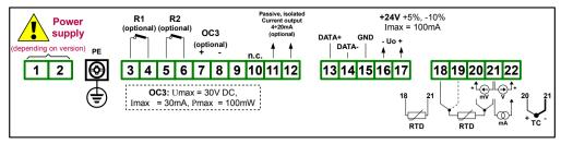
Figure 4.8. Terminals description (two relay, one OC-type and passive current outputs)
