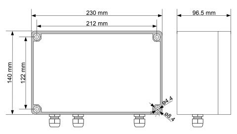
Figure 4.1. Device and assembly dimensions of the case
