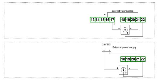
Figure 4.13. Connection of voltage converters
