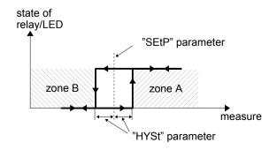
Figure 6.5. One threshold control of the relay/LED outputs
