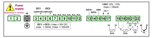
Figure 4.4. Terminals description (two OC-type outputs)
