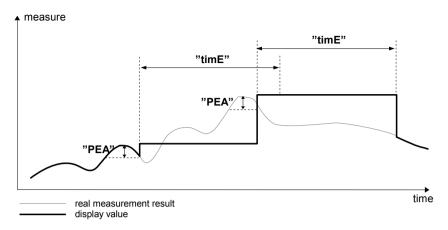
Figure 6.4. Process of peaks detection
