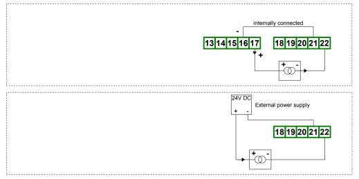
Figure 4.11. Connection of 2-wire current converters
