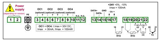
Figure 4.7. Terminals description (four OC-type outputs)
