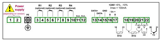
Figure 4.6. Terminals description (four relay outputs)
