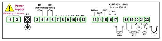
Figure 4.3. Terminals description (two relay outputs)
