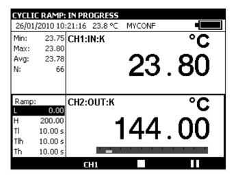
During generation of a cyclic ramp, a progress bar indicates the state of progress. The function keys are used to control generation:
