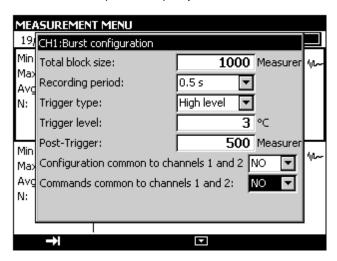
If high-level or low-level trigger is selected, the trigger level and number of data points to be stored after this trigger must be defined.
