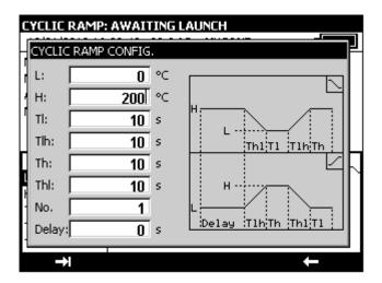
The parameters of a cyclic ramp are: B: minimum amplitude of the signal.
