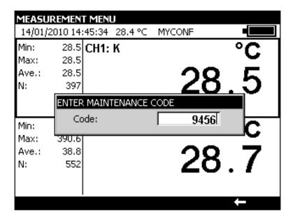
To exit the Maintenance mode, press the **End** function key.
