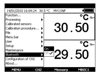
A name may be assigned to a unit connected to a Bluetooth $^{\circ}$  network with the F1 key **MENU** $\rightarrow$  **Setup** $\rightarrow$  **Bluetooth** $\rightarrow$  **Name local.**
