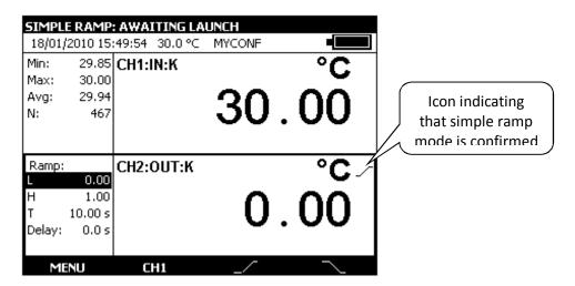
The key is used to launch an increasing ramp and the function key is used to launch a decreasing ramp.
