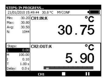
During generation of a staircase, a progress bar indicates the state of progress. The function keys control generation:
