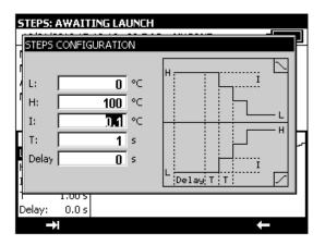
The parameters of a staircase are:
