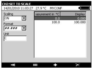
The **Define...** menu is used to program up to 10 lines of 2 values: X and Y = f(X).
