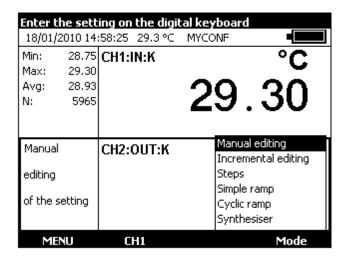
When the transmission window is open, the T150 is set by default to the Manual edit mode.
