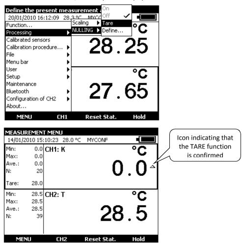
The **ZERO** → **Define...** menu is used to program the Tare value (positive or negative). This value is subtracted from the measurements:
