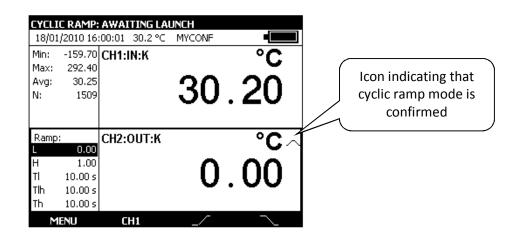
The function key is used to launch an increasing cyclic ramp and the function key is used to launch a decreasing cyclic ramp.
