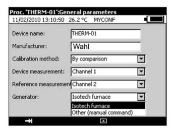
Press ENTER to confirm the options in this screen, then select the probe type for channel C2 then channel C1.
