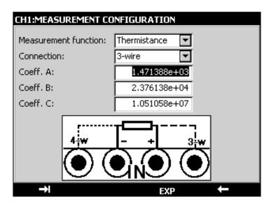
Wiring diagram is automatically detected by the calibrator. The T150 displays an icon showing the connection used to carry out measurement ( for 2 wires, for 3 wires or for 4 wires).
