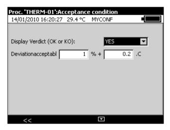
The unit may be set to display a "Verdict": "OK" or "KO" at the end of the procedure. In this case, set permissible deviation in percent and units (according to the type of measurement).
