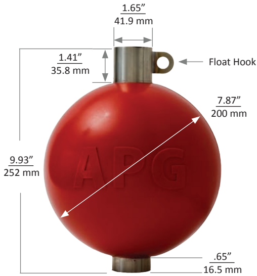
Float F - Polyurethane with 316L Stem (0.44 SG)
