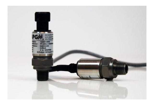
Series PT-200 0.5% Industrial Pressure Transmitters are rugged, general purpose sensors that offer reliable and accurate measurements under harsh conditions. The sensor fitting is machined from a solid piece of 17-4PH SS to provide stable operation when subjected to shock and vibration. PT-200s also incorporate digital compensation and temperature correction for high accuracy and stability.
