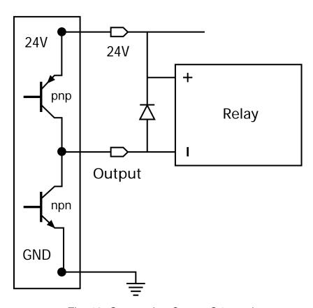
Fig. 13: Connecting Output Q1 to relay
