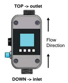
Fig. 2: Installation position of Flowmeter
