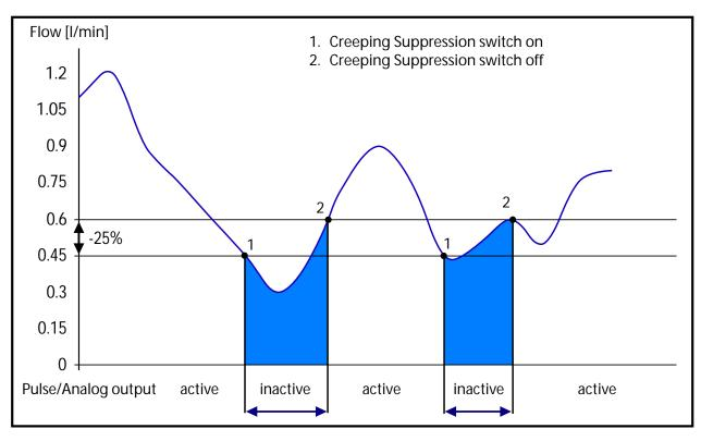
Fig. 12: Function of the creeping suppression illustrated with 0.6 l/min
