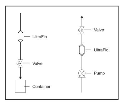
Fig. 3: Mounting examples for UltraFlo
