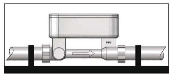
Fig. 5: Mounting the UltraFlo
